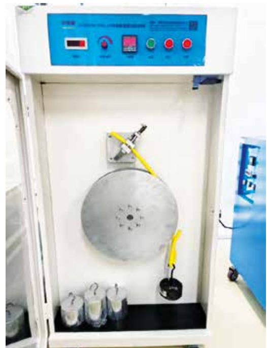
JIS C3005: 2014 clause 4.29 (abrasion) testing
