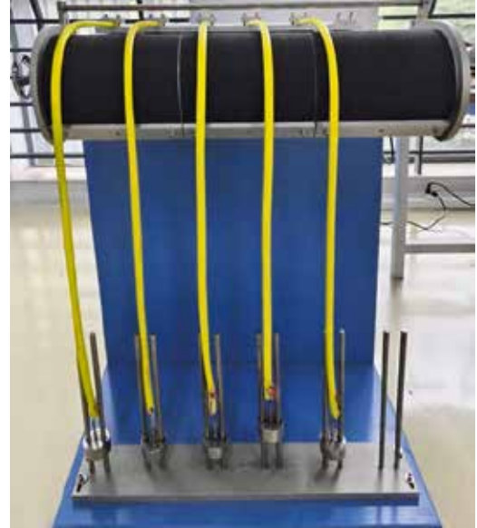
UL 2256-2021 clause 7.10 (abrasion resistance) testing
